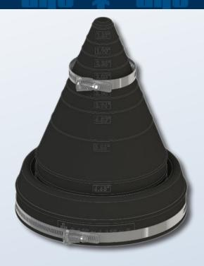
APS manufactures full, molded, conical End Seals with easy to read size indicators for versatile installation on a variety of carrier sizes. Each End Seal comes with a pair of quick adjust Stainless Steel band straps that cover all sizes within the range, so no custom-made items are needed. The End Seals are manufactured from 1/8" thick durable, chemical resistant EPDM rubber.
