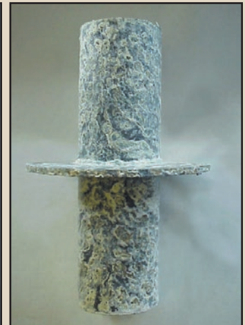
Figure 4: Galvanized Wall Sleeve after 500 hours of exposure
