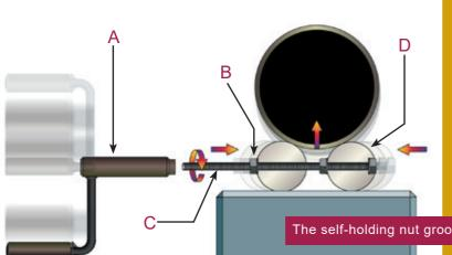
Using the installation tool (A) to tighten the hex nut (B) on the all-thread rod (C) brings the UHMW bars (D) together, which raises the pipe and allows easy inspection of the pipe. Loosening the nuts returns the rods and the pipe to its original position.
