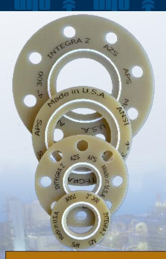
The Integra Z® gasket kit is comprised of EC-5000 material for gaskets and washers, developed and used by NASA for absolute zero operating temperature -273 °C / -459 °F. Sleeves are available in G-10 or optional Nomex materials. Metal backup washers are available in stainless steel.
