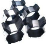
These spacers center water, sewer, gas, and other fluids in casings, offering reliable, easy-to-install alternatives to wooden skids. APS offers stainless steel band spacers and carbon steel spacers with 8" and 12" widths, sizes 3" through 120". Field changeable modular runners are also available from 1" to 6", as well as glass filled or stainless steel rollers.
