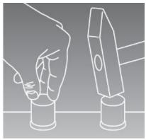
Caps may be reinstalled after initial installation. Kleergel® Corrosion Inhibitor Grease must be applied for maximum corrosion protection.
