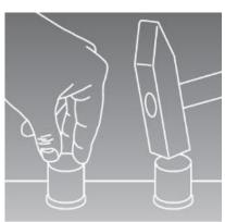
Caps may be reinstalled after initial installation. Kleergel® Corrosion Inhibitor Grease must be applied for maximum corrosion protection.
