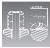
Caps must be secured onto head of bolt or nut fitting flush with the surface of the flange or substrate
