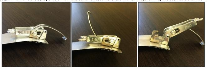
Step 2: Wrap the Spray Shield around the flange with the mesh liner down and attach the latch to the catch plate. Start with the center slot and adjust if necessary.
