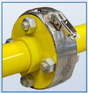
APS Splash Arrestor® is designed from a multi-layered mesh lining made of 316 Stainless Steel that provides a controlled downward disbursement of spray outs. This metal shield is resistant up to 2000°F and pressure resistant up to 3500 PSI.
